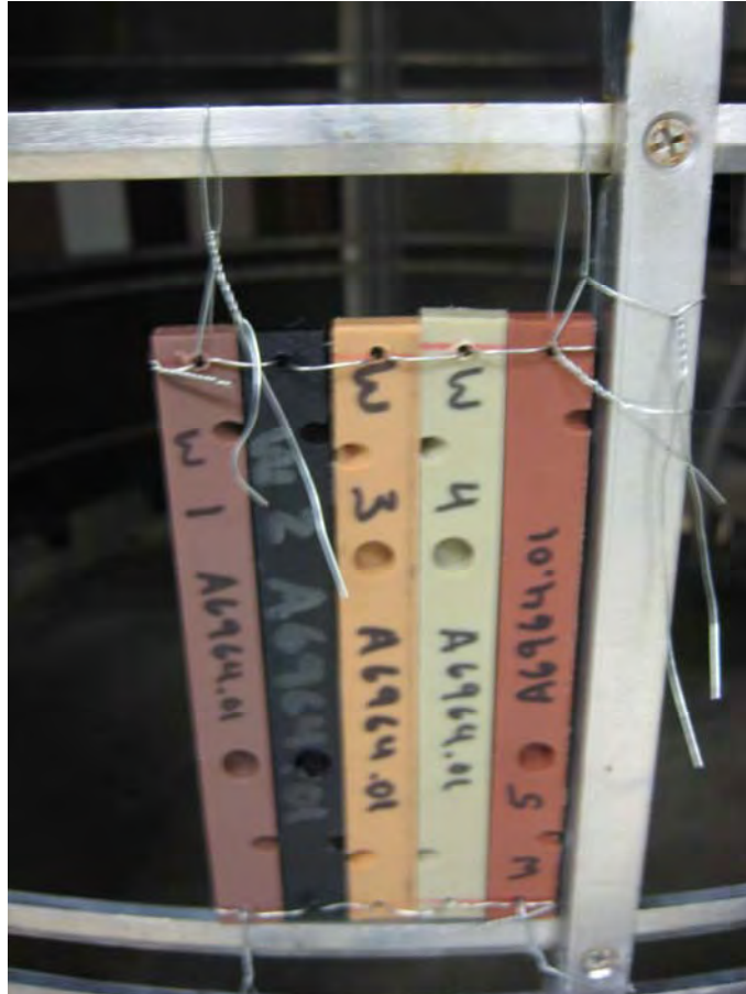
Photo No. 2 UV Resistance Testing - Specimens Installed in Artificial Weathering Machine
